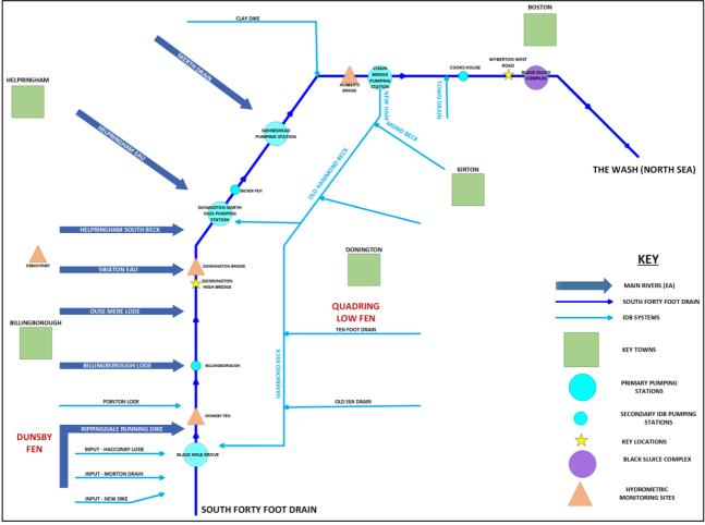
Figure 2: Schematic of all the key rivers in the South Forty Foot Drain Catchment
